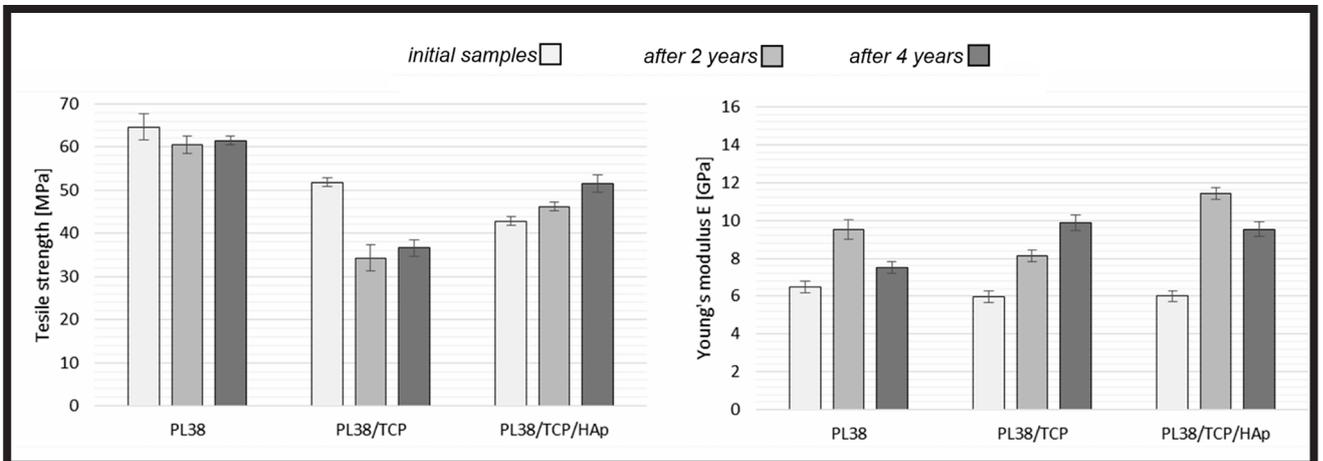
FIG. 9. Comparison of mechanical test results ( $R_m$  and  $E$ ) of the “R” type fixation miniplates of the initial samples, after 2 and after 4 years.
