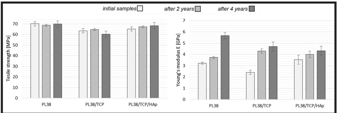
FIG. 5. Comparison of average R<sub>m</sub> and E values obtained during mechanical testing of dumbbell-shaped specimens of the initial samples, after 2 and after 4 years.
